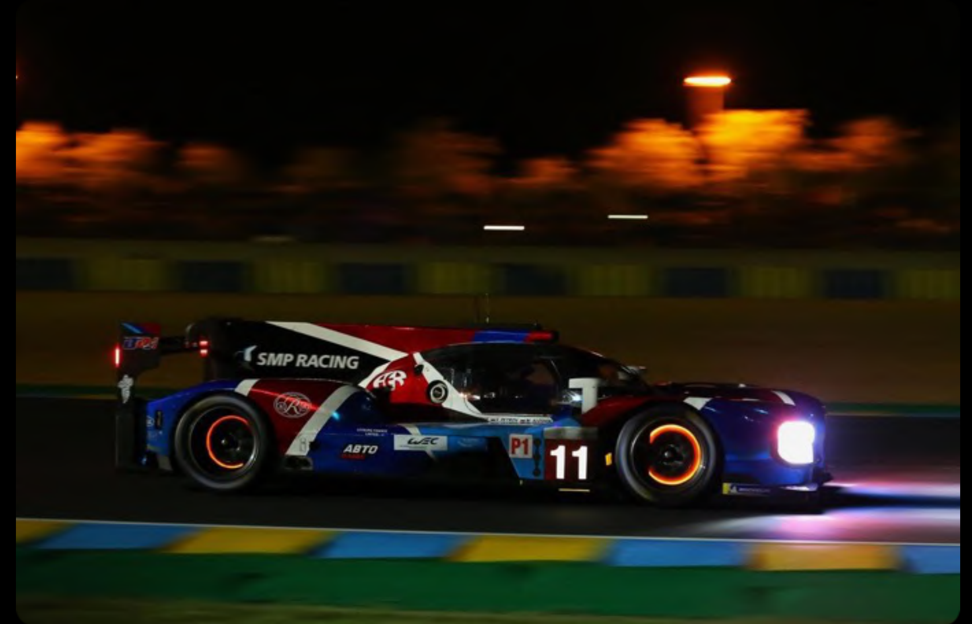
Figure 6: Hot brakes radiate a large amount of heat into the wheels and tyres. (SMP Racing)
